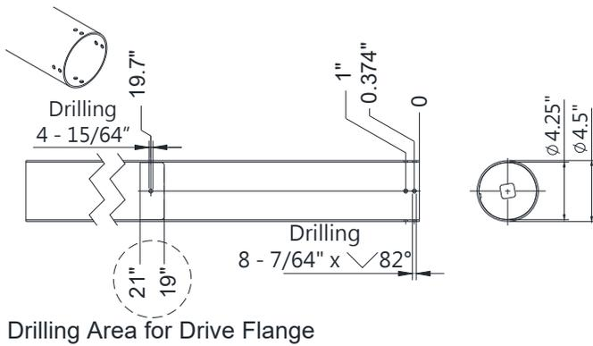
1.2 Pipe end mounting and drive flange mounting illustrations.
