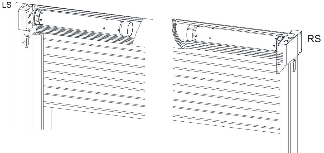
**NOTE:** Any change in mounting position may result in a change of operator rotation and consequently in a change of control functions. Consult factory for any changes. (LS mounting position is LH operator, RS position is RH operator)
