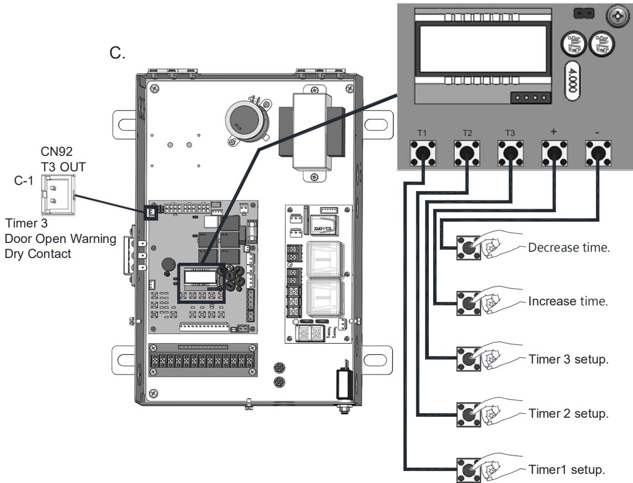
1. T1 – Mid-open timer: Timer starts counting when door leaves close limit. Door stops after opening for set time. Pressing open again at mid-open position will cause door to open to open limit.
