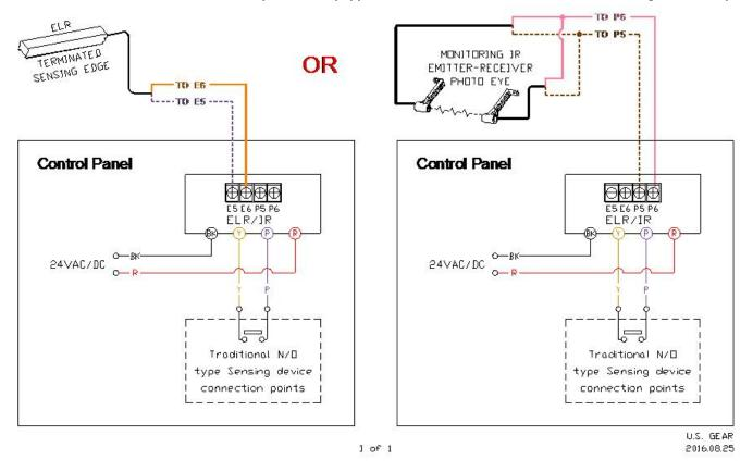
The **GW-40-59-TRA-A01** device enables monitored sensing devices to be connected to "legacy" motor operators that is designed to use non-monitored NO sensing devices. It is designed such that in any condition where the adaptor does not detect a properly working monitored sensing device the indicator LED will go out and the output relay contact will close and initiate a fault reaction in the operator.
