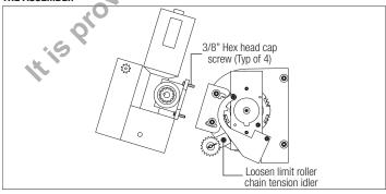
Loop limit roller chain around limit switch sprocket on motor operator and tension idler sprocket on bracket. Do not pull limit roller chain taut at this time. Loop the drive chain
