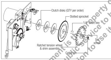
Install the clutch disks onto the 3/4" diameter shaft. Install the slotted sprocket, spacer, 1/4" shaft key and ratchet tension wheel as snown. Faster the coffer pin in the end of the 3/4" shaft, to secure the components from moving laterally. Tighten all set screws on the door sprocket and inner set collar. Verify that the clutch disks rotate freely. Orient the clutch disks and slotted sprocket as shown below:
