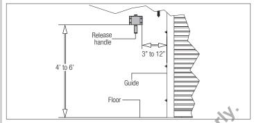
While individual installation locations may vary depending on site conditions, there commended location is shown in the illustration. Determine where the release handle assembly will be installed and attach it to the wall using the fasteners provided. Again, be sure to choose a location that is convenient to operate and will avoid interference with the chain hoist operation and any obstacles that may be in the path of the cable routing.
