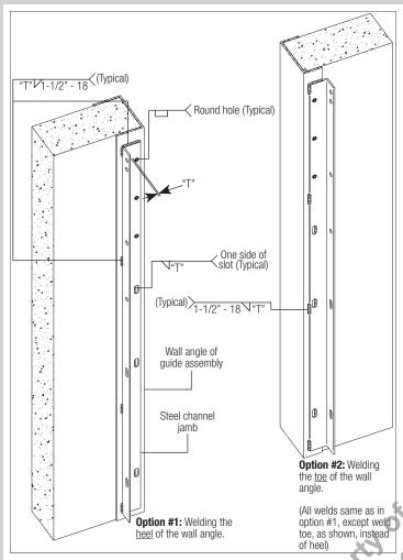
Use E6010 / E6011 electrodes or electrodes of equivalent strength. All welding must be done "vertical up" (i.e. starting the individual weld bead and welding upwards). Use fillet welds based on the information provided above.
