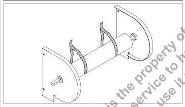
Using a chain hoist, fork lift, sling or some means of lifting, determine the balance point of the barrel assembly with the brackets mounted on it.
