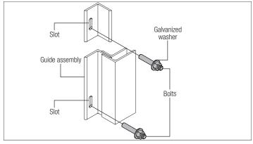
IMPORTANT: FIRE DOORS WILL TEND TO EXPAND DOWNWARD. IT IS NECESSARY TO SET THE GUIDES OFF THE FLOOR THE REQUIRED EXPANSION CLEARANCE PER THE INSTALLA-TION DRAWING PROVIDED AND INSTALL THE GUIDE BOLTS AT THE BOTTOM OF SLOTS.
