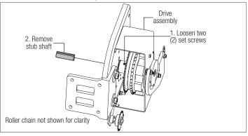
After removing the stub shaft check to make sure that a square key is still visibly in place
