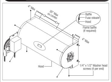
Hoods over 14' long require the use of intermediate support(s). For hoods equipped with a flame baffle, the supports go outside the hood. These are bolted to the hood using screws from the inside of the hood. Raise the front hood and set over the flanges on the bracket assemblies. Fasten hood to brackets using the 1/4" diameter self-tapping washer head screws provided. Fasten hood securely to the wall using the fasteners listed on the hardware bill.
