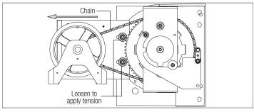
Adjust chain until slack is between 1/4" and 1/2", as shown in the illustration below. If the chain slack exceeds 1/2", re-cut roller chain.
