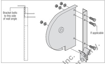
**IMPORTANT:** INSTALL BRACKET BOLTS FROM INSIDE SO THAT NUTS ARE ON OUTSIDE OF WALL ANGLE TO KEEP BOLTS FROM INTERFERING WITH CURTAIN.
